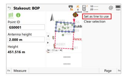
This new option ensures that when needing to change the reference line, the ongoing field task is not interrupted by avoiding the need to change panels or stop the measurement process.
