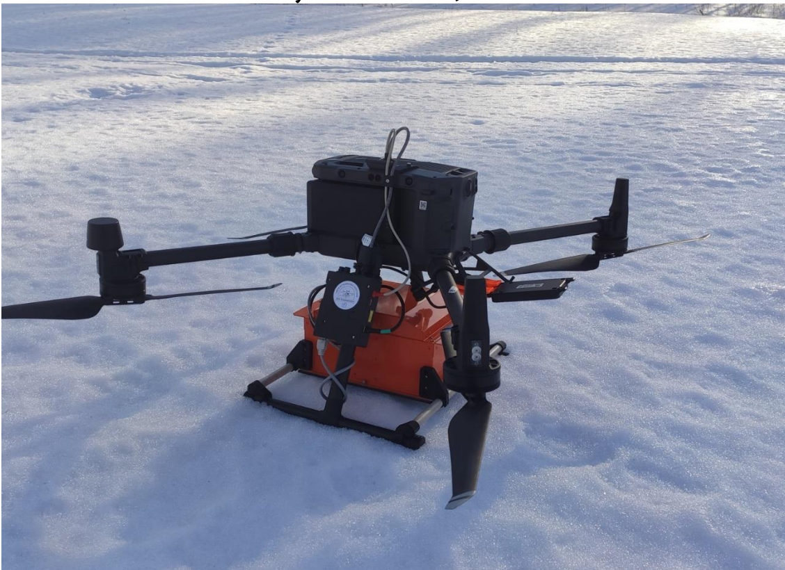
Zond Aero 1000 NG GPR system under DJI M300 RTK drone:
