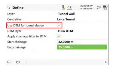
When **Use DTM for tunnel design** is checked, the DTM layer can be viewed or selected. The DTM data can be filtered by chainage, which reduces the amount of computation needed, which can help improve performance when using very large tunnel designs.
