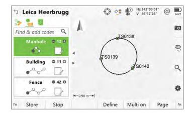
Note that because auxiliary points are used to construct the 3 pt rectangle, 2 pt and 3 pt circles, the line used to represent the shape will not be linked to the measured points within the database. This means that the geometry of the line will not be editable once the shape is completed.
