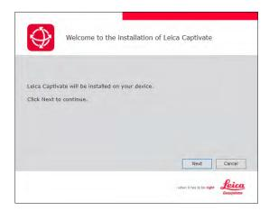
When manually upgrading the tablets from previous versions to Leica Captivate v8.00, a message will first ask you to manually un-install the former 32-bit version of Leica captivate. This step is not needed if the upgrade to Leica Captivate v8.00 is done using the **Online update** option from the **Update Software** panel.
