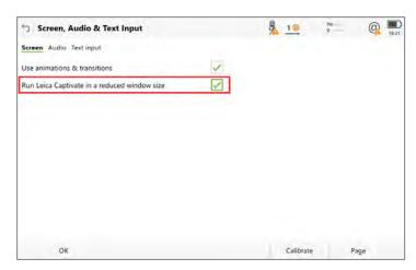
In Leica Captivate v8.00, a new setting has been added that allows Leica Captivate to run in a reduced window size. The **Run Leica Captivate** in a reduced window size setting can be found in the **Screen, Audio & Text Input** panel. After enabling the setting, a message requests that Leica Captivate needs to be restarted for the change to take effect.
