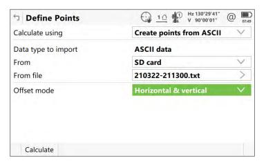
The COGO Rail tool also offers the possibility to select the offset mode, which defines in which plane the offsets should be applied. The offsets can be applied and calculated with respect to **Horizontal & vertical**, or with respect to the design cant of the track using the option **With super-elevation**.
