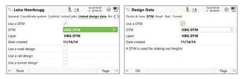
Once a DTM job is selected, the new setting **Use DTM for tunnel design** will be available in the **Define** panel of Stake or Check Tunnel.
