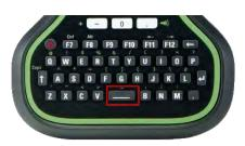
When selecting linework in the **Select Linework** panel, a search can be used by pressing an alphanumeric key on the keyboard, for example, pressing the B key would start a search for items beginning with "B". With the item found, the required option needs to be confirmed to be selected. Previously, this would require two button presses; one to confirm and select the search and one to close the panel.
