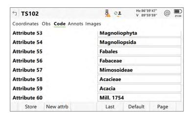
With Leica Captivate v8.00, it is now possible to define up to 60 attributes per point code. The attributes for each code in the codelist can be pre-defined in the Leica Infinity Code Manager or created on-the-fly when measuring in Leica Captivate. Import and export options that previously supported 20 attributes will now support 60 attributes.
