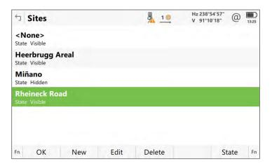
A new filter icon in the left upper corner of the **Home** panel indicates the visibility of jobs in the job carousal. The job visibility can be filtered by site, by memory device or both. If any filter is active, the icon is shown green. The filter is active when the state of any site is set to hidden, or the jobs are filtered by storage device.
