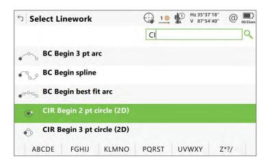
With the three new linework options, the new way to access the **Select Linework** panel and confirm the search result, a huge improvement in efficiency can be gained whilst measuring with linework. With these improvements, it is possible to save between 4 and 7 key presses per measured object, reducing the time to collect data in the field.
