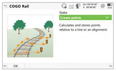
The tool offers similar calculation methods to the equivalent tool in COGO Road (Number of points, Chainage increment and Single point), however the COGO Rail tool offers a new calculation method called Create points from ASCII. An ASCII data file can include any number of 'points' which are defined by chainage, offset and height in a simple, delimited format. The file can be imported and a batch of COGO points calculated and created.
