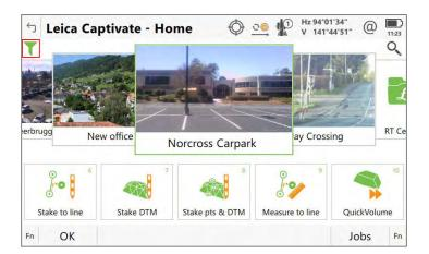
Clicking on the icon opens the **Filter** panel which allows defining which filters should be applied to the jobs shown in the **Home** panel.
