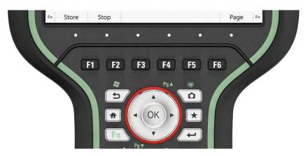
From Leica Captivate v8.00 onwards, the **Store** and **Stop** button position has been changed. Now, when continuous distance measurements are being used, **Store** is assigned to the **F1** function key, and **Stop** assigned to the **F2** function key. This means the **OK** button on the keyboard can also be used to store points, making measurements more intuitive and comfortable.
