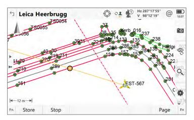
Note that when using other distance measurement modes, such as **Once** (single shot), the key assignment has not been changed. **Measure** remains on **F1** and **Store** remains on **F3**, meaning the **OK** button can still be used to make single measurements.
