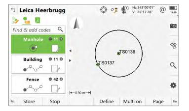
**3 pt circle (2D)** - using this linework option, a circle can be created by measuring three points on the circumference of the circle. The first measured point will define the height of the circle. Only three points will be exported, and other auxiliary points used to construct the shape will be hidden from view.
