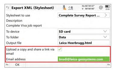
Once the **Upload a copy and share a link via email** setting is checked, a single email address can be entered. When the data is exported in the selected format, the data is additionally uploaded to a Hexagon cloud service and an email is sent to the defined recipient containing a link to the data.
