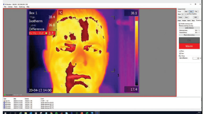
The thermal image shows the hot spots in the corner of the eyes.
