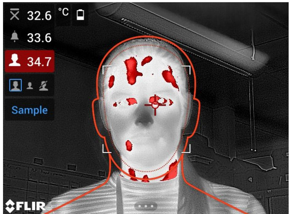
The basics of the screening function is to first build up a base of reference temperature samples. When a person is screened, the camera compares the measured temperature with the average of the reference samples. If the camera detects an elevated temperature, an alarm will trigger.
