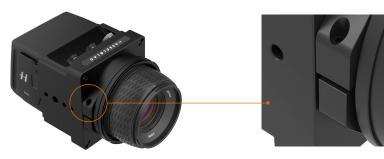
Insert the supplied 2.5mm Allen key into the bolt and rotate clockwise half a turn to engage the lens mount lock.
