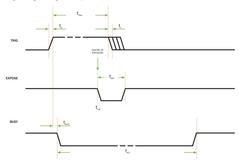
The electrical timing when using **EXPOSE** signal as full indicator:
