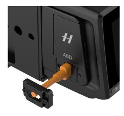
Attach the lock part and tighten the screws using the supplied 1.5mm Allen key. Note that it needs to be oriented correctly to fit.
