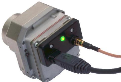
**Figure 5: VPC Physical Connections**
