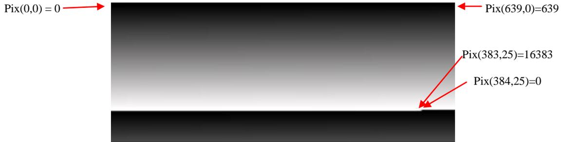
**Figure 17: Ramp test pattern example for Top Portion of Ramp Image**
