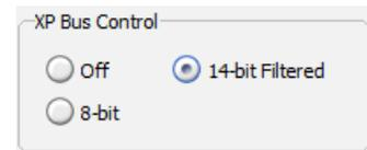
**8-bit:** Data is provided after application of the current Automatic Gain Control (AGC) and Dynamic Detail Enhancement (DDE). The 8-bit data is essentially a digital version of the same data provided on the analog video channel, but CMOS data does not include symbology. With the Tau 2.4 release LUTs and digital E-Zoom are user selectable.
